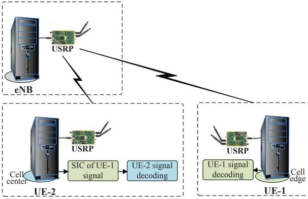
Fig. 1. Deployment scenario of SDR-based NOMA system.
