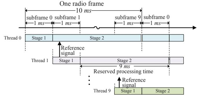
Fig. 3. Multi-thread processing method for UE receiver.
